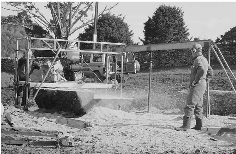
Large portable mill working on a huge 'grand-daddy' pine (65+ yrs old)
